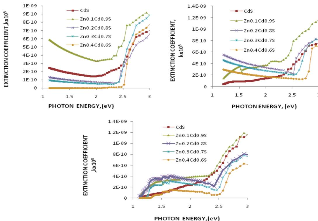
FIG.8. Extinction Coefficient of thin films for 30 min, 45 min and 60 min.
