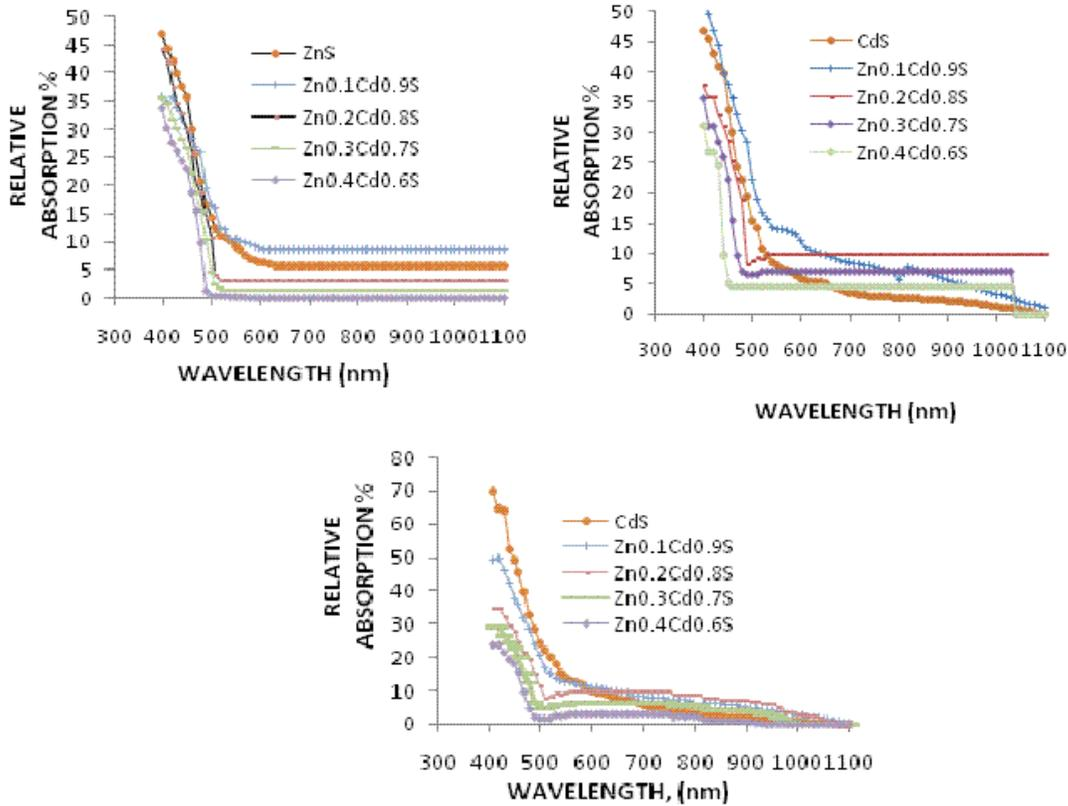
**FIG. 4.** Absorption Spectra of thin films for 30 min, 45 min and 60 min.
