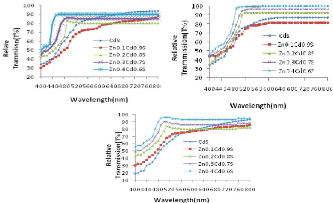
FIG.1. Transmittance of films for 30min, 45 min and 60 min depositions
