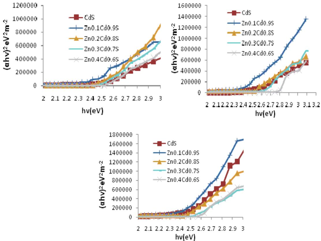
FIG. 2. Energy band gap for 30 min, 45 min and 60 min depositions.
