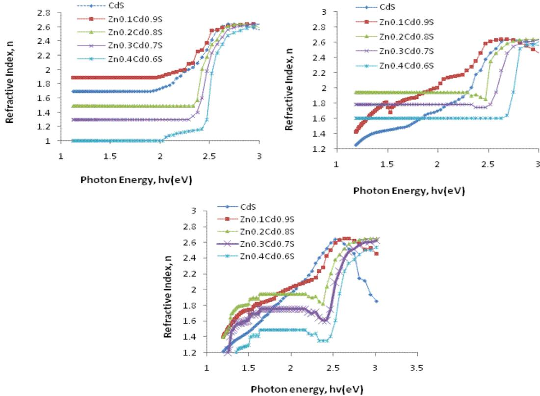
**FIG. 6.** Refractive Index of thin films for 30 min, 45 min and 60 min.
