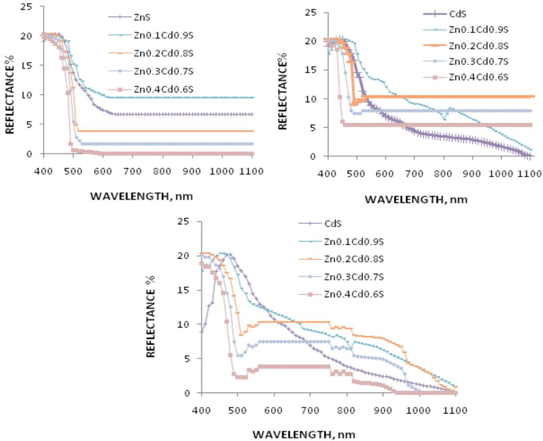
**FIG. 5.** Reflectance Spectra of thin films for 30 min, 45 min and 60 min.
