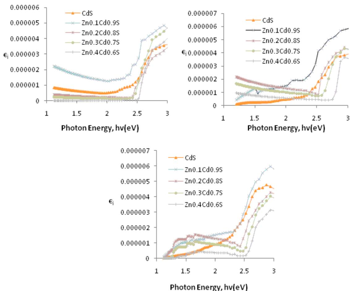
**FIG. 10.** Imaginary Dielectric Constant of thin films for 30 min, 45 min and 60 min.
