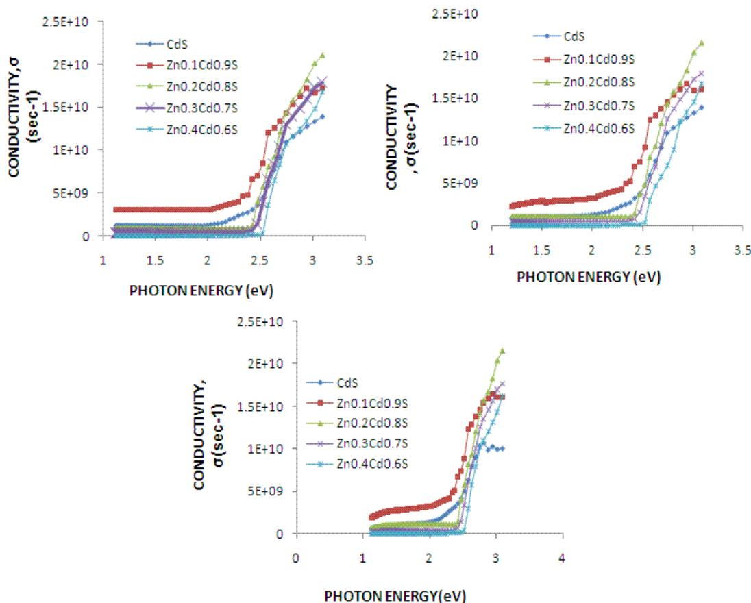
**FIG. 7.** Optical Conductivity of thin films for 30 min, 45 min and 60 min.
